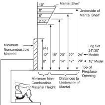
Figure 6 - Minimum Mantel Clearances Without Using Hood
